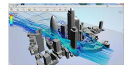
Flow Design can quickly model wind behavior around closed buildings and provide an understanding of where there may be risks of elevated velocities and/or stagnant regions.
