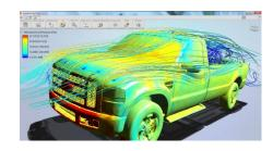
In automotive applications Flow Design shows regions where air will recirculate, provide an understanding of the size and location of the wake region, and identifies high and low pressure regions on the body, and approximates the drag force and coefficient.
